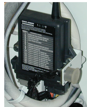
Crane Control Receiver
