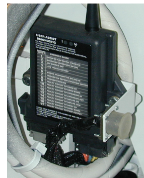
Crane Control Receiver
